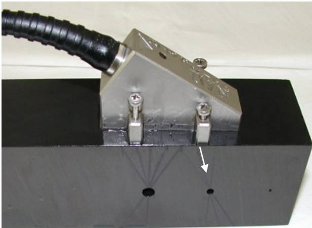
Angle beam (12°) insonification of side drilled hole \varnothing 3 mm
