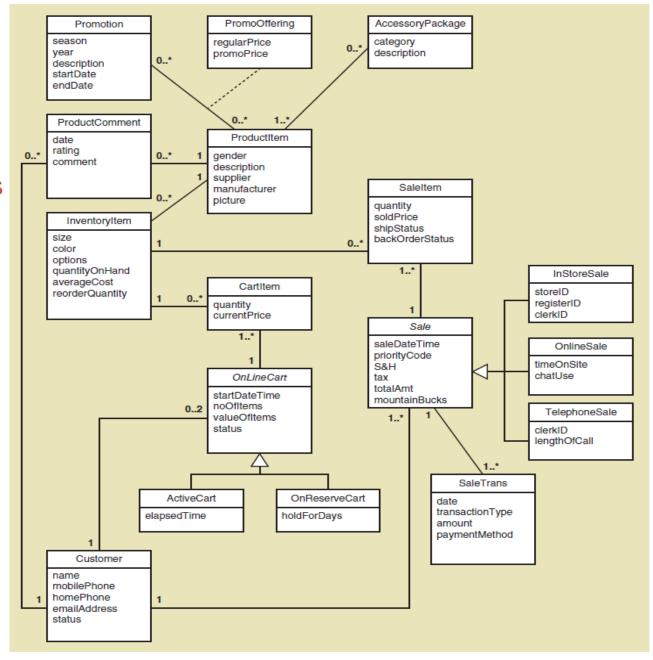
RMO CSMS Project Customer Account Subsystem Domain Model Class Diagram
