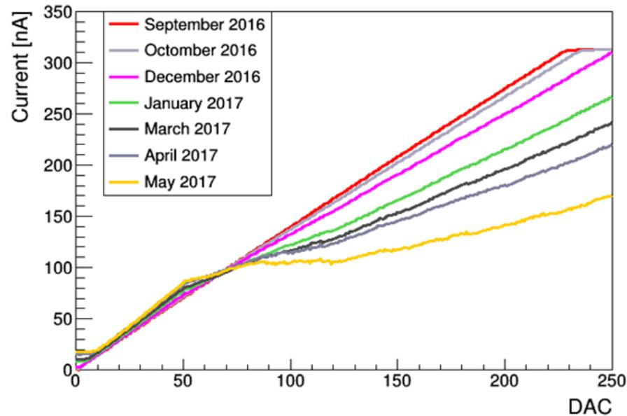
DAC SCAN of VCASN for A4W7G7R38 at the first stages of irradiation tests
