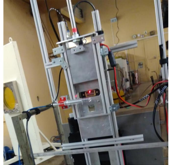
Positioning stage with connected ALPIDE chip
