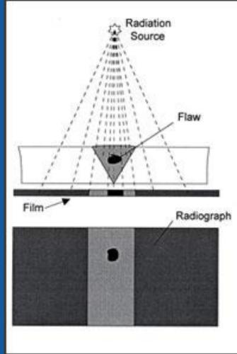
To be a usable film, the area of interest (weld area, etc.) on the film must be within a certain density (darkness) range and must show enough contrast and sensitivity so that discontinuities of interest can be seen. These items are a function of the strength of the radiation, the distance of the source from the film and the thickness of the part being inspected. If any of these parameters are not met, another exposure ("shot") must be made for that area of the part.
