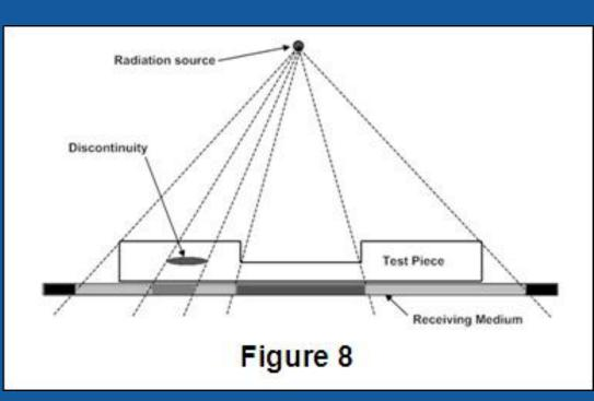
Gamma radiation is given off by decaying radioactive materials, with the two most commonly used sources of gamma radiation being Iridium-192 (Ir-192) and Cobalt-60 (Co-60). IR-192 is generally used for steel up to 2-1/2 -3 inches, depending on the Curie strength of the source, and Co-60 is usually used for thicker materials due to its greater penetrating ability.
