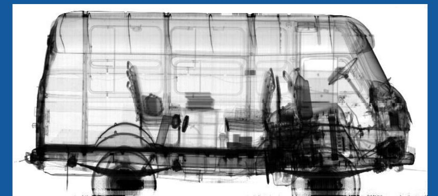
The CT image is developed from multiple views taken at different viewing angles that are reconstructed using a computer. With traditional radiography, the position of internal discontinuities cannot be accurately determined without making exposures from several angles to locate the item by triangulation. With computed tomography, the computer triangulates using every point in the plane as viewed from many different directions.
