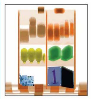
This technique uses a reusable, flexible, photostimulated phosphor (PSP) plate which is loaded into a cassette and is exposed in a manner similar to traditional film radiography. The cassette is then placed in a laser reader where it is scanned and translated into a digital image, which take from one to five minutes. The image can then be uploaded to a computer or other electronic media for interpretation and storage.
