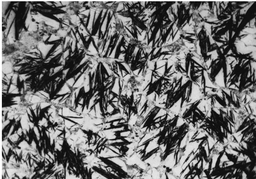
Figure 10.13 Photomicrograph of martensitic microstructure. The needle-shaped grains are the martensite phase, and the white regions are austenite that failed to transform during the rapid quenching. \times 600
