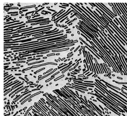
Figure 10.7 Photomicrograph of a eutectoid steel; the pearlite microstructure consists of alternating layers of \alpha ferrite and Fe_3C . \times 500
