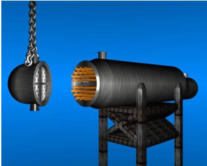
STRATCO contactor reactor for sulfuric acid alkylation
