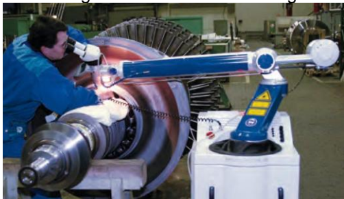
Fig. 3. Mobile Laser Welding
