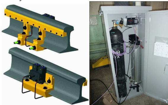
Figure.1. Node of lubricating device and cabinet.
