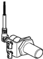
Fig. 4. Capacitive proximity sensors
